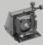
Mount, 3-axis, modified for this setup to hold a glass retrosphere
